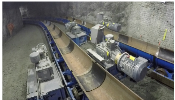
The shuttle-with-bypasses configuration balances need for high throughput with light infrastructure requirements and narrow drift width.
